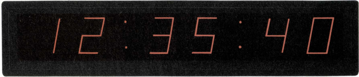
MAN6 — .6" high, the MAN6 looks an inch high from across the room. The complete, gapless font makes all ten digits and nine letters unmistakably clear. It should find application in many instruments, consumer electronics, and cockpit displays.
