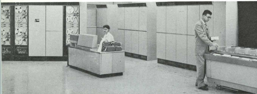
Multiple FR-400 tape transports installed in a GE-100 data-handling system. The GE-100 will provide high-speed, accurate, automatic processing of bank accounts and transactions.
