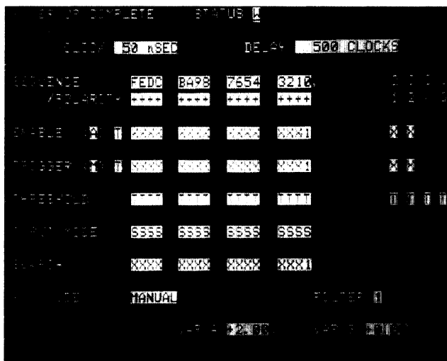
Figure 3.14. Status W reflects the fact that the clock period has been changed to 50 ns.
